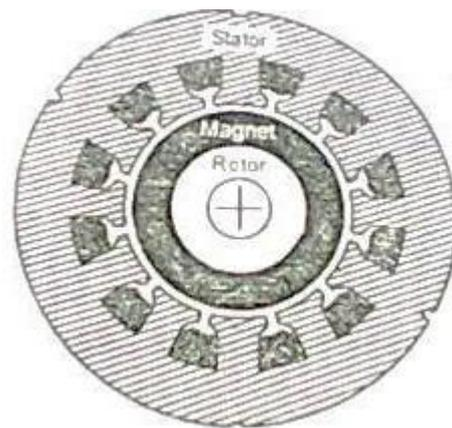
**Figure 2.1.1 construction of BLPMD motor**
